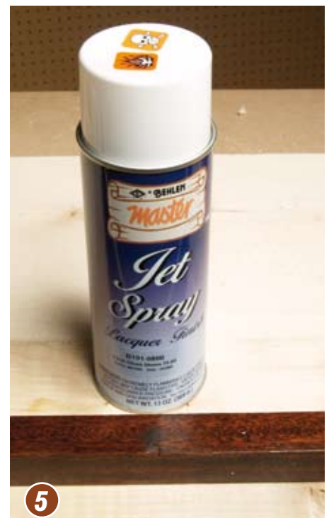
5 After filling I sprayed the area, as advised, with a quick flash of top coat Behlen lacquer
