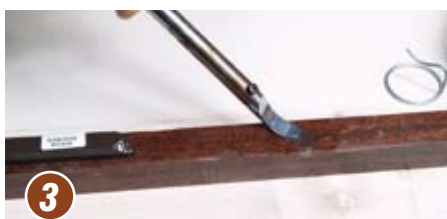
3 Burn-in Balm is very effective and used to surround the filled area. The spatula is stroked over the fill to level it. Normally the fill material that is drawn to the edges of a hole would stick to the surrounding area but the balm prevents adhesion and also protects the original surface from heat damage
