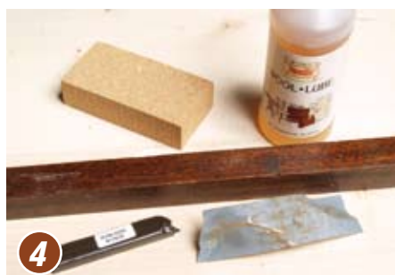
4 The spatula and the surface are then cleaned with a rag before the fill is flattened with 400-grit paper and the Wool Lube lubricant, also very effective
