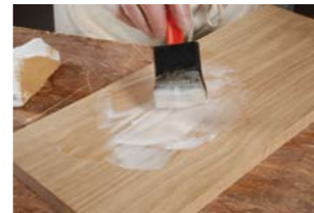
Water-based grain filler is applied to open-grained oak...
