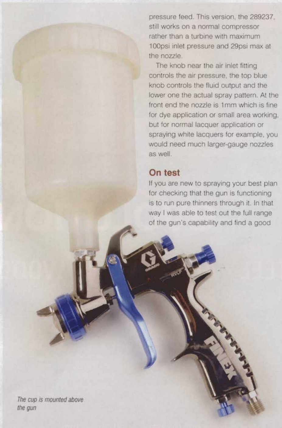
The top blue knob controls the fluid output and the lower one the actual spray pattern
