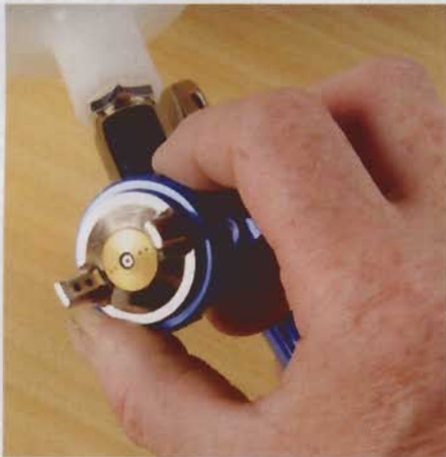
The top blue knob controls the fluid output and the lower one the actual spray pattern
