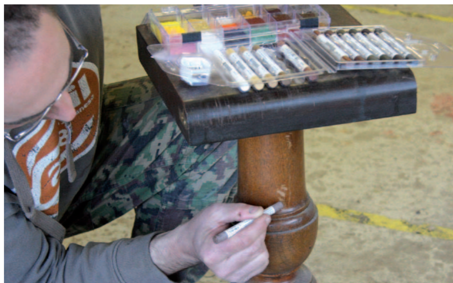
Repair A dent like this on the pedestal table is an ideal candidate for some work with the Bendal Sticks from Mohawk
